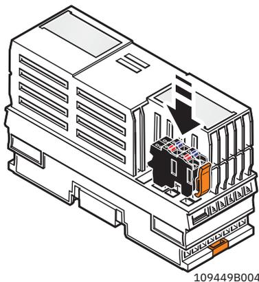
Supply the SPLC 1000 (together with the PLCnext Control used) with an external 24 V DC voltage supply. The permissible voltage range is 19.2 V DC to 30 V DC (ripple included).
