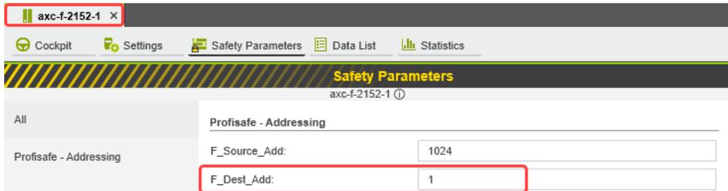
Bild 3-5 F-Addresses of the F-Host (RFC 4072S) and F-Device (SPLC 1000)
