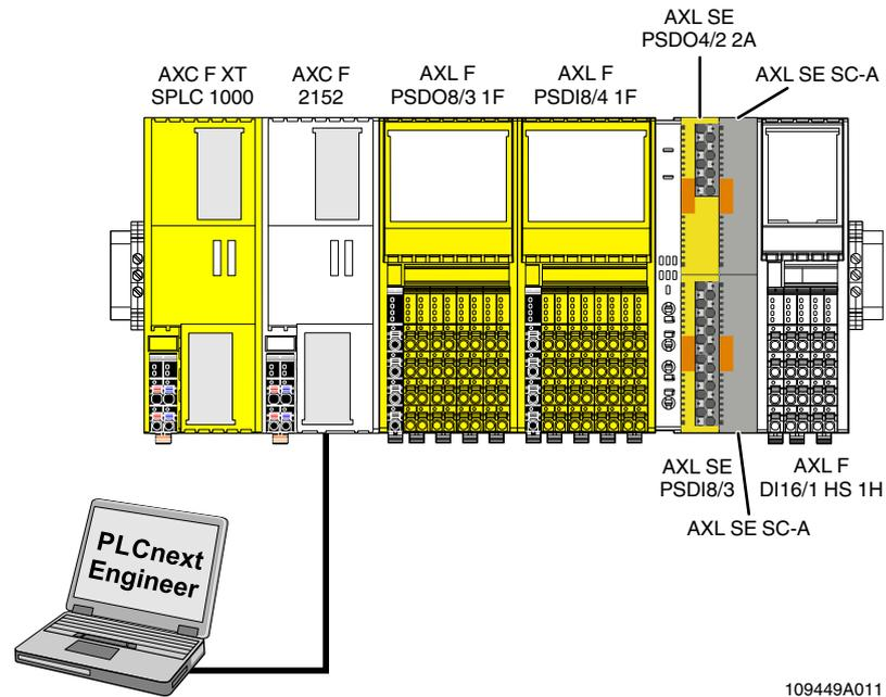
In this example configuration, the SPLC 1000 is aligned to the left of the modular AXC F 2152 small-scale controller in an Axioline F station.
