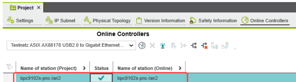
Figure 6-9 Successful assignment of the configured controller to an online device
