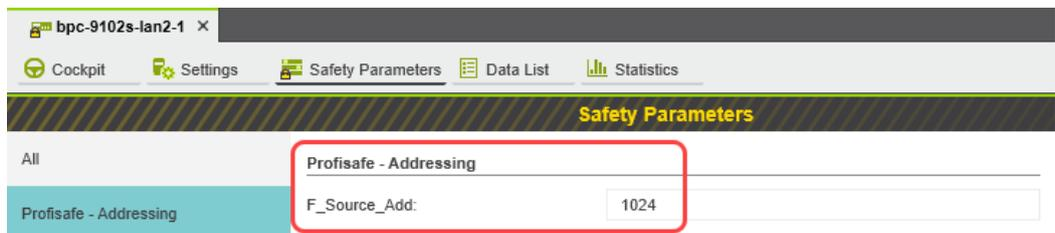
Figure 6-31 F-Address of the F-Host: F\_Source\_Add (F\_Source\_Address)
