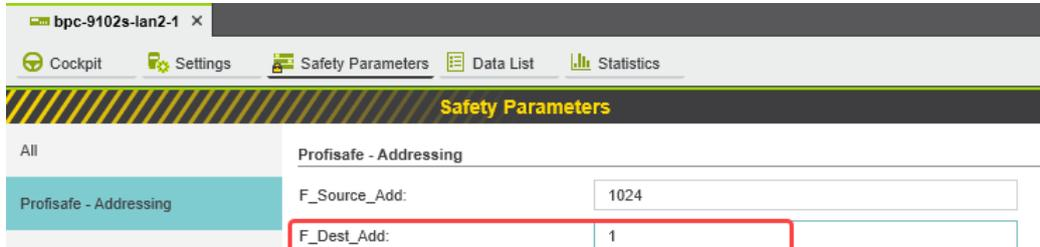
Figure 3-4 F-Address of the SPLC 3000 F-Device in PLCnext Engineer: F\_Dest\_Add (F\_Destination\_Address)
