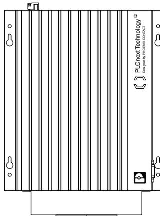
Figure 4-2 Mounting position of the BPC 9102S
