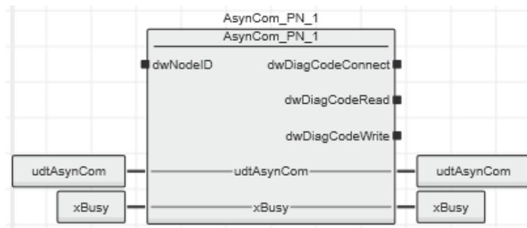
Figure 7-1 `AsynCom_PN_1` function block
