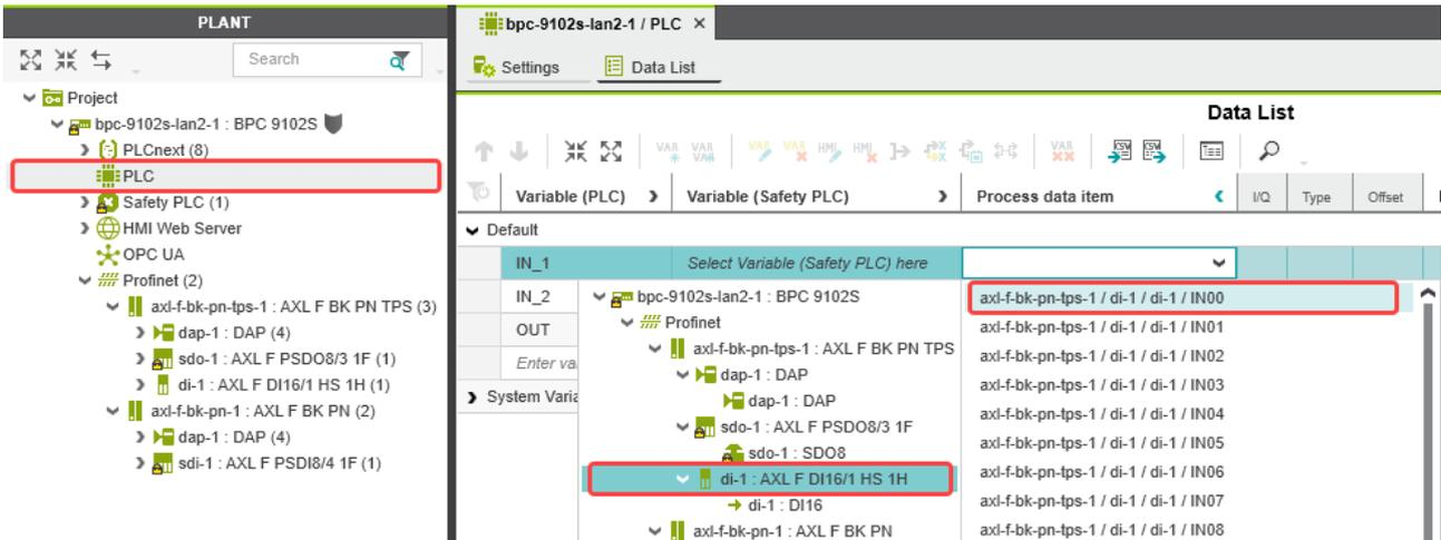
Figure 6-29 Assigning process data
