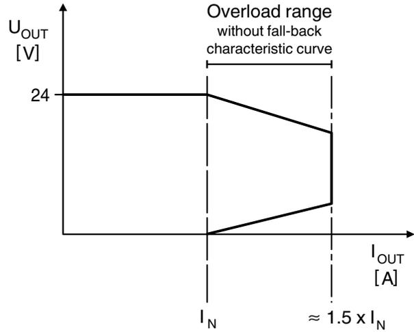
Figure 5-2 Overload range **without** fall-back characteristic curve
