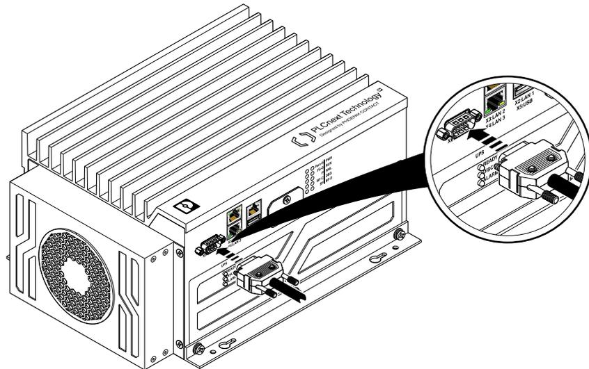
Figure 4-6 Connecting the COM service interface of the BPC 9102S
