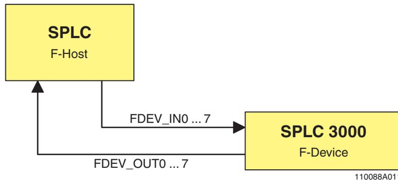
Figure 3-3 Data exchange between the F-Device of the SPLC 3000 and the higher-level F-Host
