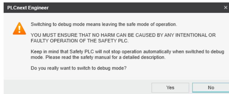
Figure 6-56 Exiting safe mode – switching to debug mode
