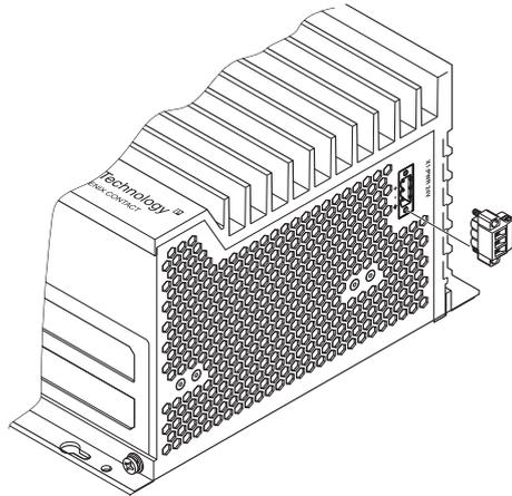
Figure 5-3 Connection of the supply voltage
