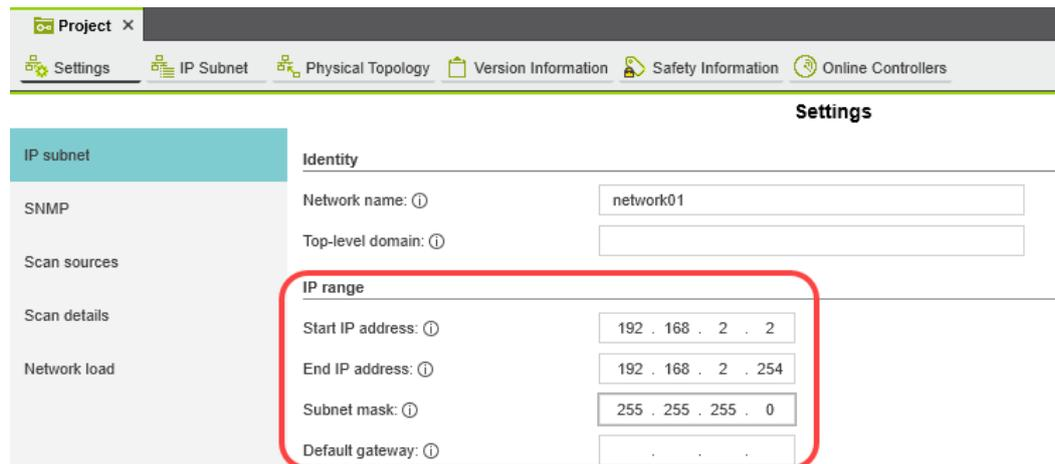
The screenshot shows the 'Settings' window in PLCnext Engineer. The 'IP subnet' tab is selected. The 'IP range' section is highlighted with a red box. The values are as follows:
