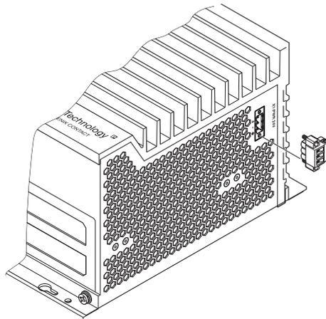
Figure 10-1 Removing the power supply
