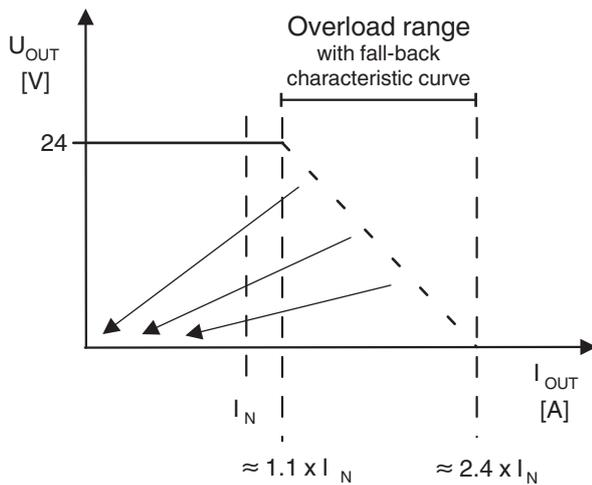
Figure 5-1 Overload range **with** fall-back characteristic curve
