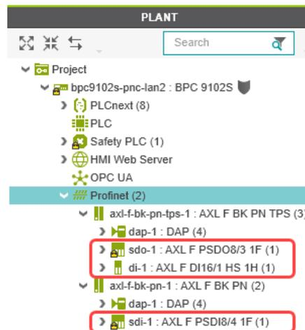
Figure 6-22 I/O modules () in the example project
