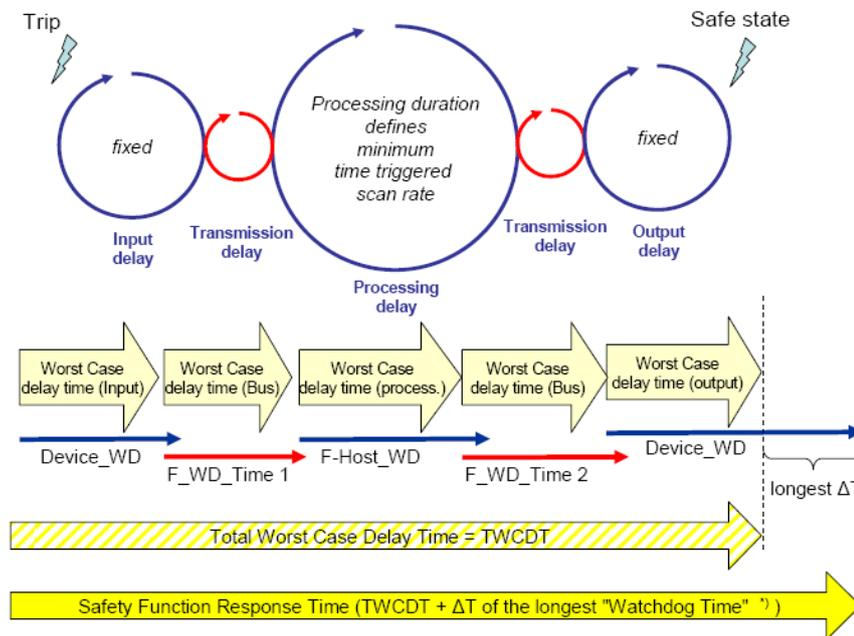
Figure 3-6 Calculation of the SFRT response time
