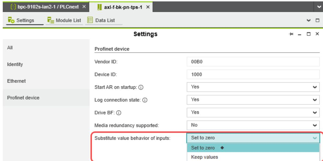
Figure 13-3 PROFINET device – “Substitute value behavior of inputs”
