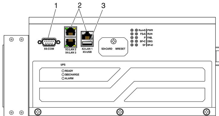
Figure 3-16 Interfaces of the BPC 9102S
