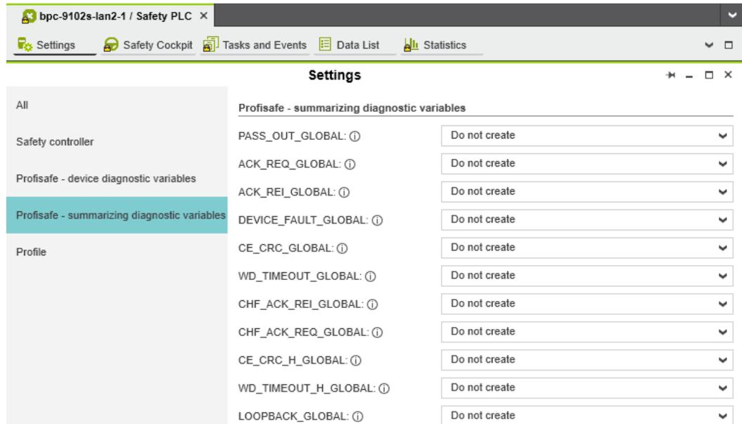
Figure 6-36 Management/diagnostic variables for all configured F-Devices
