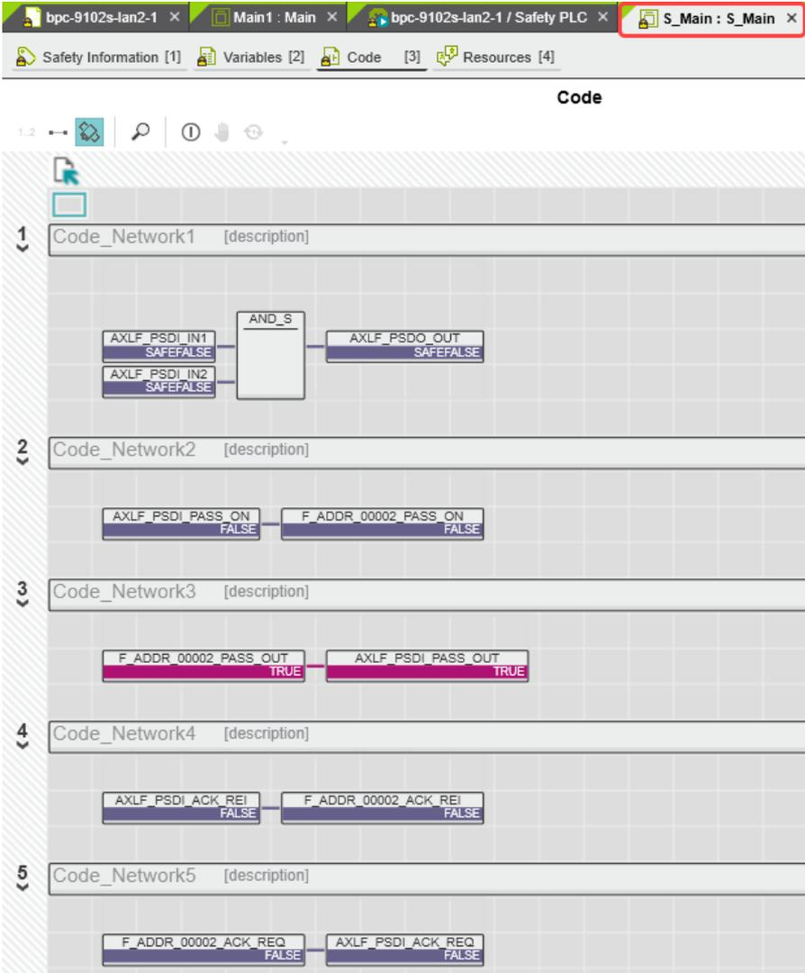
Figure 6-58 PLCnext Engineer – Passivated PROFIsafe F-Devices
