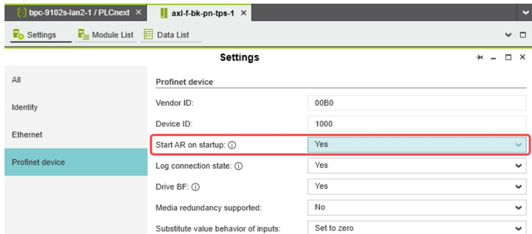
Figure 13-1 PROFINET device – “Start AR on startup”
