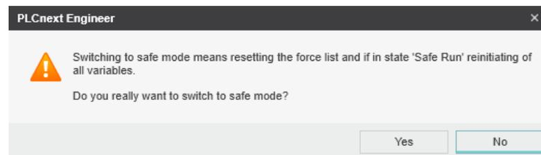
Figure 6-57 Exiting debug mode – switching to safe mode
