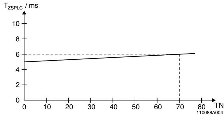
Figure 3-10 Cycle time of the SPLC 3000 ( $T_{ZSPLC}$ )
