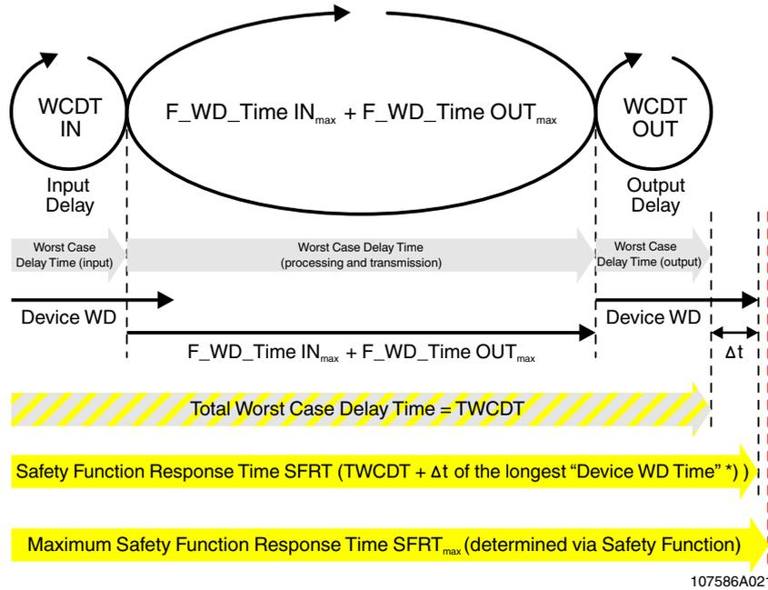
Figure 3-7 Simplified calculation of the SFRT response time
