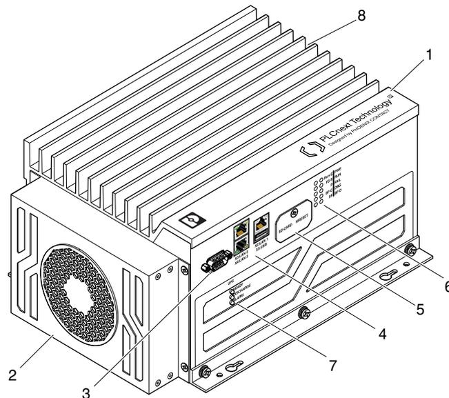
Figure 3-13 Connection and operating elements as well as test marks and security seals of the BPC 9102S
