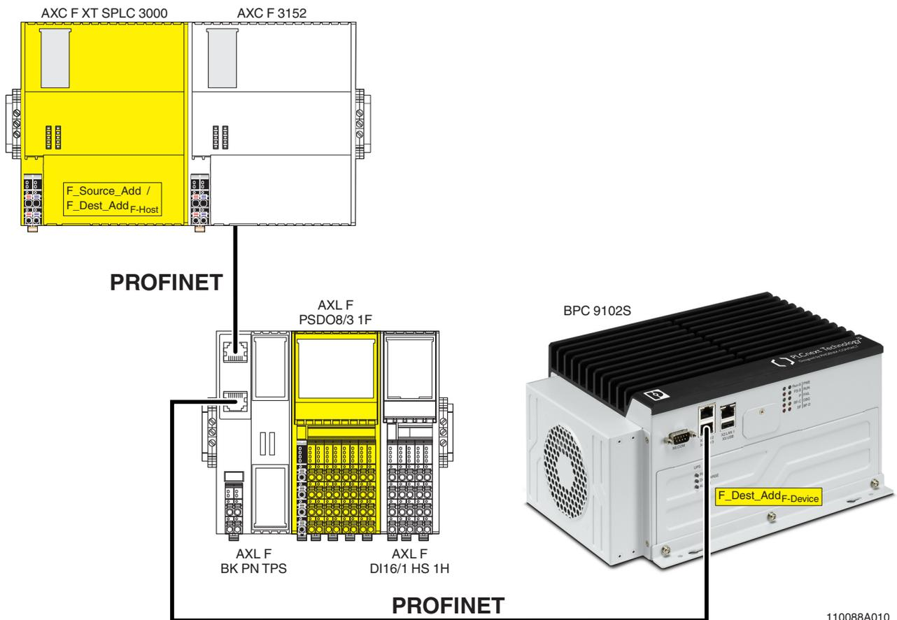
Figure 3-5 F-Addresses of the F-Host (SPLC 3000) and F-Device (SPLC 3000)
