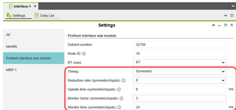
Figure 3-9 “Settings” editor of the interface editor group of the PROFINET device (settings of the AXL F BK PN TPS PROFINET bus coupler)
