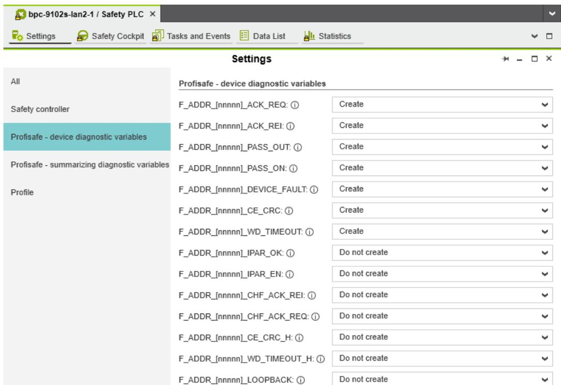
Figure 6-35 Management/diagnostic variables for each configured F-Device
