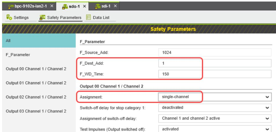
Figure 6-33 “Safety Parameters” editor: AXL F PSDO8/3 1F
