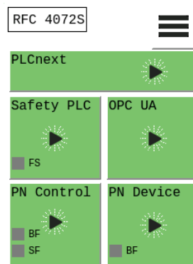
Figure 2-16 Diagnostic indicators in the home menu (LEDs)
